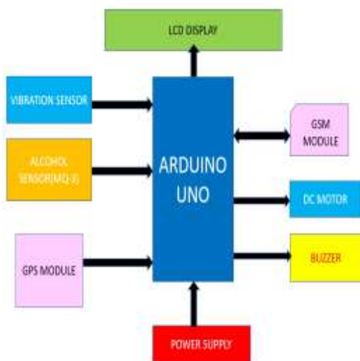
Figure 1: Block diagram of Collision Alert and Preventing System
